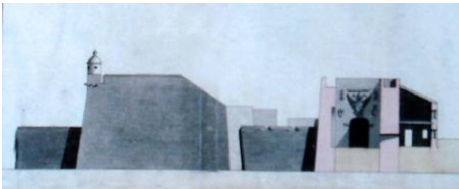
Fig 5: 1700, South Bastion and Southport Gate showing the bartizan or guerite , a small watchtower, at the SW corner of the bastion.
